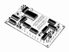
The TD-2 provides five latching on-off functions and up to 12 momentary outputs. This means, for example, that you can control a repeater and autopatch, three other latching functions such as sub-audible tone activation, and several momentary functions. Latching outputs can drive solid-state circuits directly, sinking up to 50mA, or they can drive small relays to switch power loads. The 12 momentary outputs provide a standard 5V logic output.
